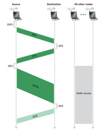
CSMA/CA Carrier-Sense Multiple Access with Collision Avoidance
